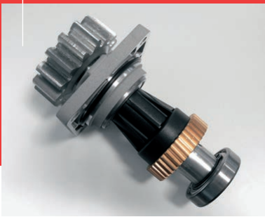
Motor shaft in steel and bronze
